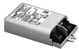
Driver (CC) - DALI - 20 W - IP20 - 700 mA max A32691-DA
